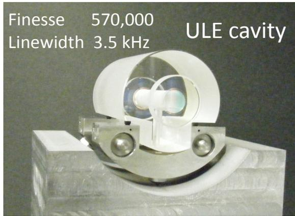
Vibration insensitive optical cavity with cut-out design: (NPL) Webster *et al.*, PRA 75, 011801 (2007)
