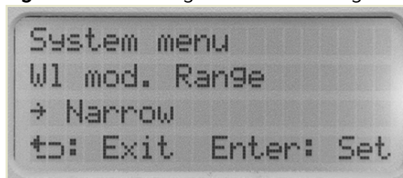
Figure 26 Wavelength modulation range set to Narrow
