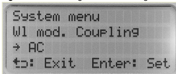
Figure 25 Wavelength modulation signal coupling set to AC
