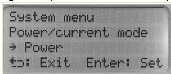
Figure 27 Operation mode set to constant power mode
