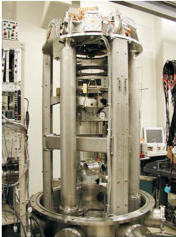
Figure 7.2: TAMA SAS prototype tower, located in the vacuum tank.
