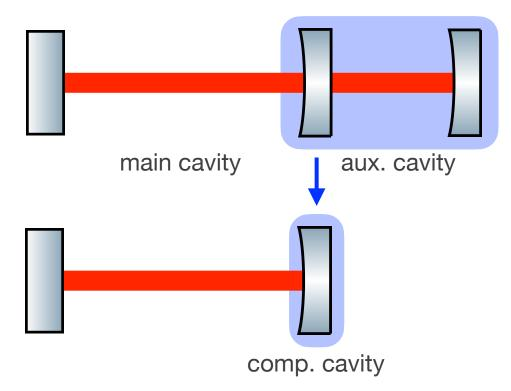
How can we understand cWFS if we take the aux.cavity a a compound mirror?
