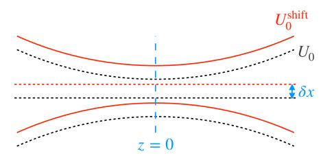
$$\begin{split} U_0^{\text{shift}}(x,z) &= U_0(x,z) + \frac{\delta x}{w_0} U_1(x,z) \\ U_1^{\text{shift}}(x,z) &= U_1(x,z) - \frac{\delta x}{w_0} U_0(x,z) \end{split}$$
