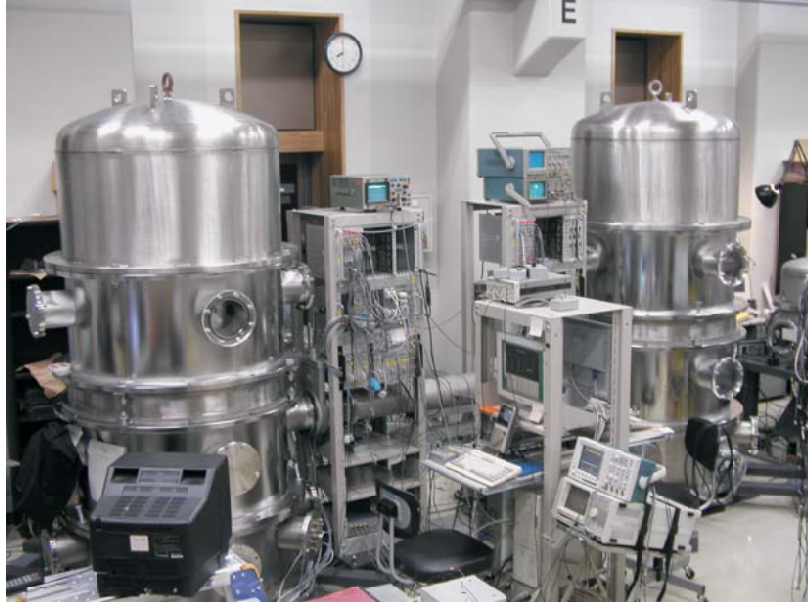
Figure 7.1: 3m Fabry-Perot cavity in the laboratory. Each vacuum tank contains one prototype SAS tower. The racks between the tanks house the electronics for the local control.
