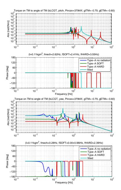
Figure 5.1: The transfer functions from the torque on the test mass to angle of the test mass(top: pitch, lower: yaw). The blue curve shows the mechanical transfer function in the absence of radiation pressure. The green and red curve show the opto-mechanical transfer functions of the soft mode and hard mode.
