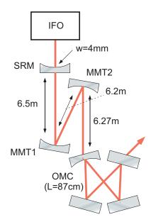
Figure 2.32: Output mode-cleaner system.
