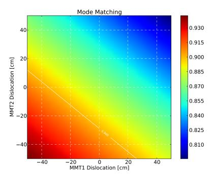
Figure 9.2: Input mode matching of iKAGRA, mapped by changing the positions of the IMMT mirrors from the optimized ones for bKAGRA.
