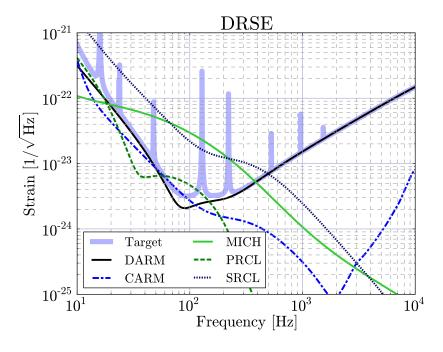
Figure 3.4: Loop Noise Coupling: DRSE
