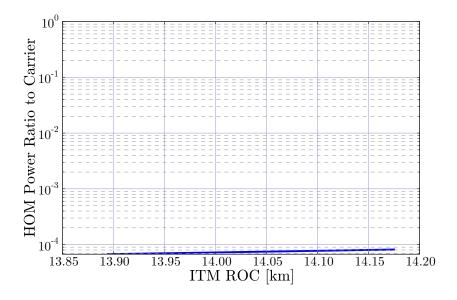
Figure 2.6: The maximum HOM power ratio in the AC as a function of ITM ROC error for the positive g-factors. The ROC is swept by  $\pm 1\%$  around the nominal value.
