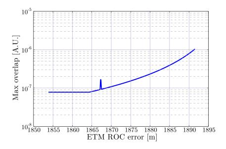
Figure 2.12: Figure of merit of the overlap between the RF SB harmonics and the HOMs when the ETM ROC is swept. g-factor is negative.
