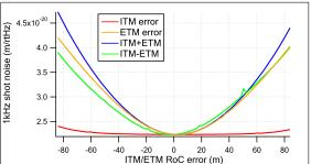
Figure 2.33: Left: Signal loss due to the differential RoC errors of the test masses, and Right: Shot noise increase due to the junk light caused by the differential RoC errors of the test masses.
