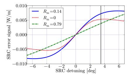
Figure 2.16: SRCL error signals for three different values of  $R_{\rm m}$ . The horizontal axis is the detuning of the SRC in terms of the one-way phase shift. The vertical axis is the signal from the POP port demodulated at the f1 frequency. The vertical line shows the operation point of DRSE (3.5°).
