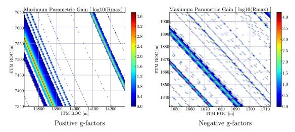
Figure 2.15: Maps of the maximum parametric gain as functions of the ROCs of the test masses. Left: positive g-factor, Right: negative g-factor. The ROCs are swept by  $\pm 2\%$  of their nominal values. White areas correspond to  $R_{\rm max} < 1$ .
