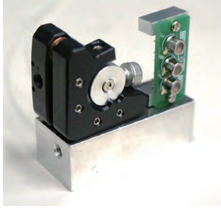
Figure 4.13: The picture of the sensor module. The left one is the fiber collimator mounted on the half inch mirror mount, and the right one is the photo sensor.
