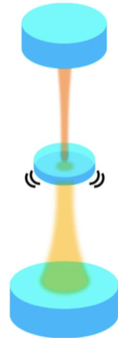
Schematic of the sandwich type optical levitation.
