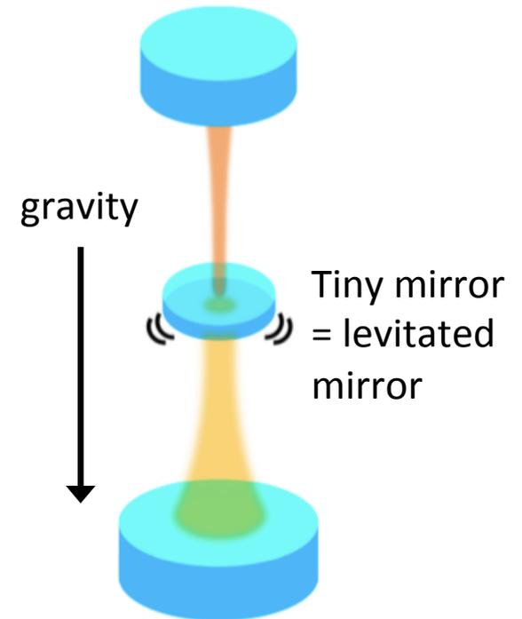
Schematic of the sandwich type optical levitation.
