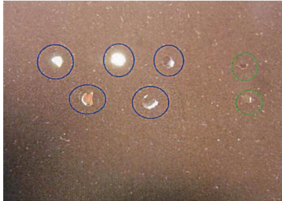
Picture of the mirror after coating. Only one of seven does not have any lack.
