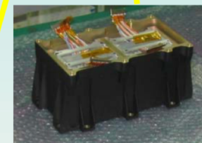
Two Torsion Antenna Modules assembled
