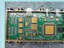
FPGA (Digital Filter) and SpaceWire I/F
