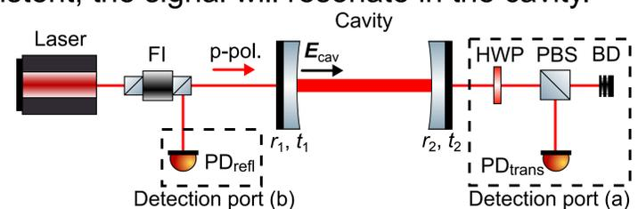
Fig. 2: Schematic of experimental setup for axion search with a linear optical cavity. Signal is detected in detection port (a) and (b). Components for phase measurement are not shown. The polarization of incident light is arbitrary if only it is linear polarization.
