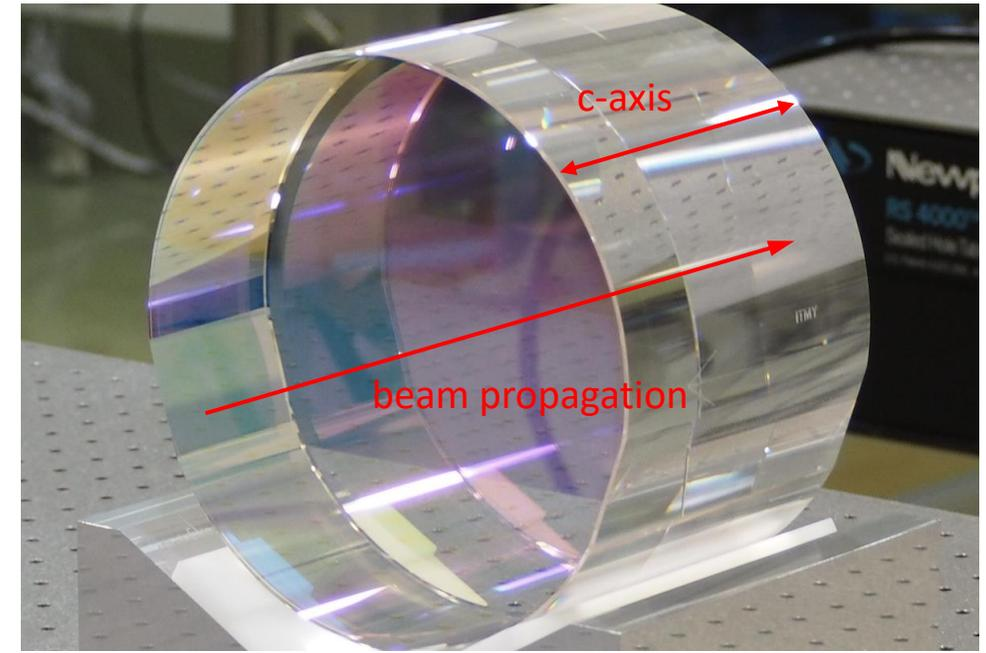
The beam propagation is aligned with the c-axis (no birefringence).
