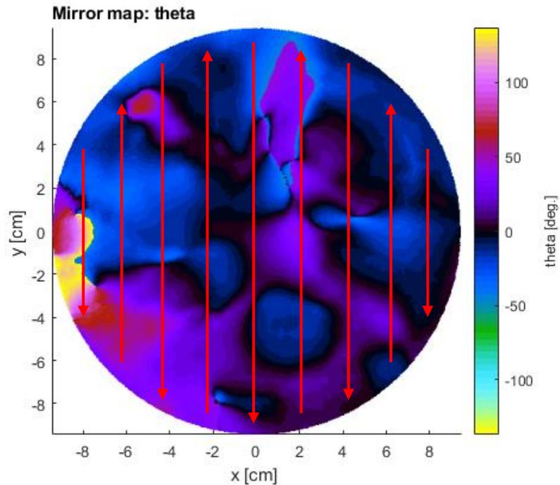
Expand the map to one-dimension and calculate the "roughness".
