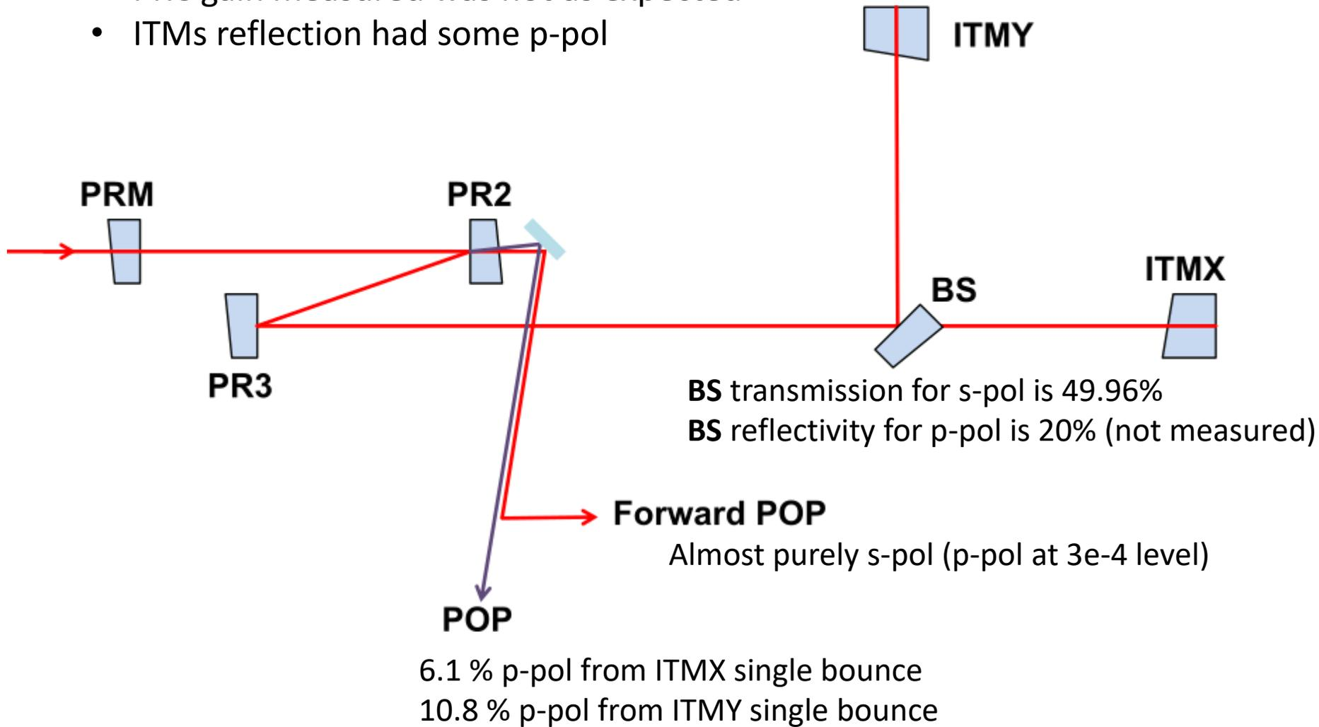
A portion of input light in s-pol is converted to p-pol.
