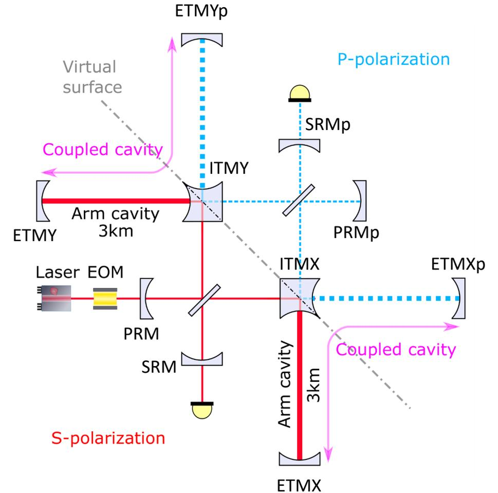
The key of the two-world approach is to define a birefringent component that defines the coupling between s-pol and p-pol light.
