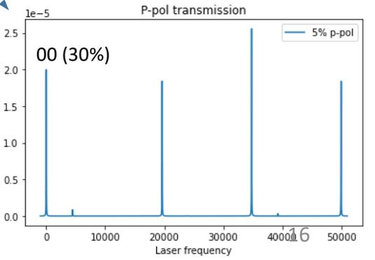
\* The difference between 1.26% (calculation) and ~1.36 (simulation) is because in the calculation we don't consider the HOM effect of p-pol. HOMs create different birefringence power from the TEM00 mode.
