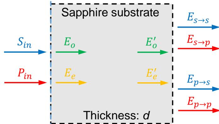
Considering the incident beam is **pure s-pol**. It is projected to e-axis and o-axis. After a propagation of thickness  $d$ , the two fields are
