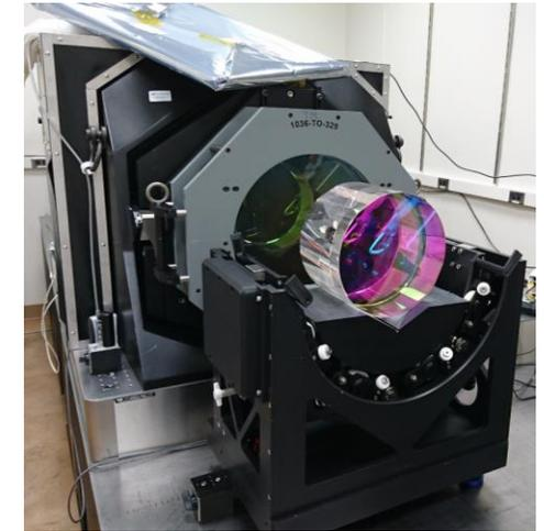
Measure TWE with different input polarization directions
