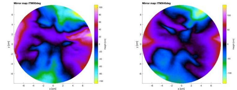
Gravity induced deformation of ITMX + astigmatism of reference sphere
