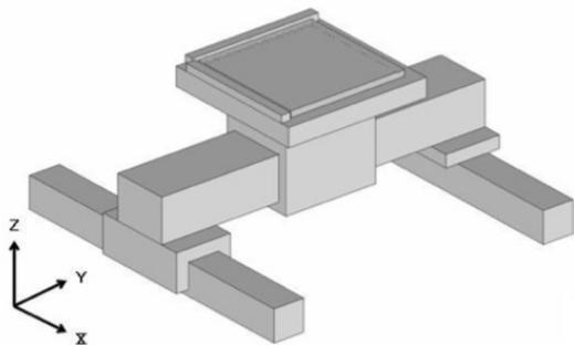
Fig. 1 Structure of XY gantry stage.
