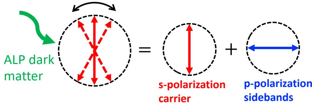
Axion signal is produced as p-polarization
