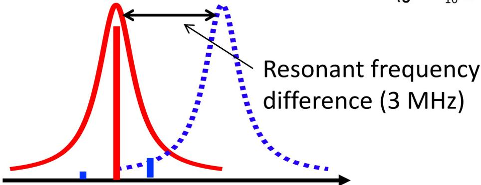
Simultaneous resonance is necessary for high sensitivity
