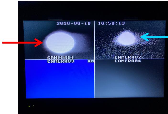
Transmitted light of auxiliary laser (p-pol.)
