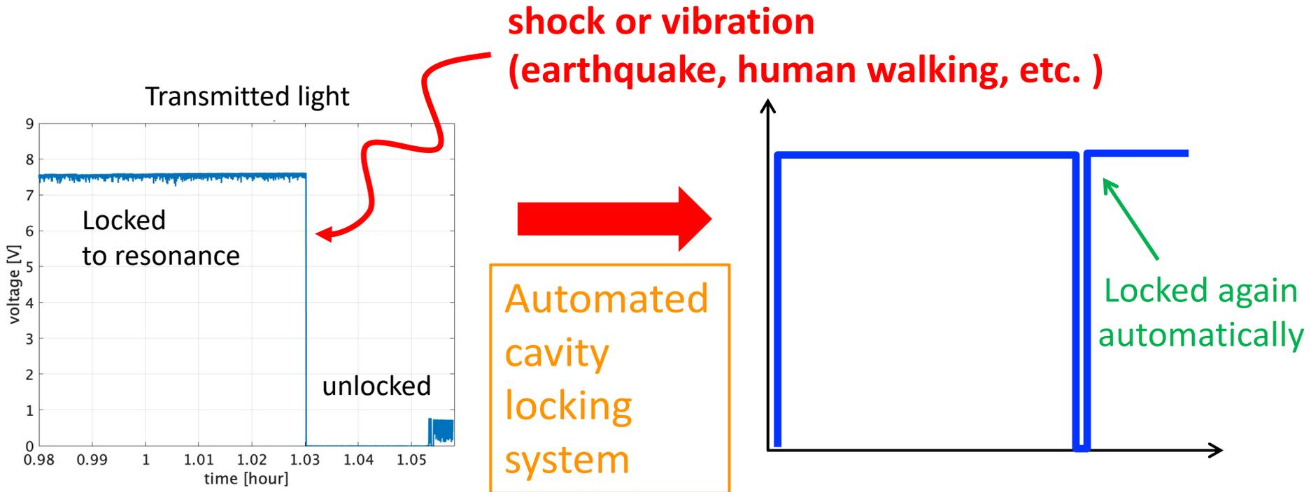
Cavity can be relocked automatically during long-term observation.
