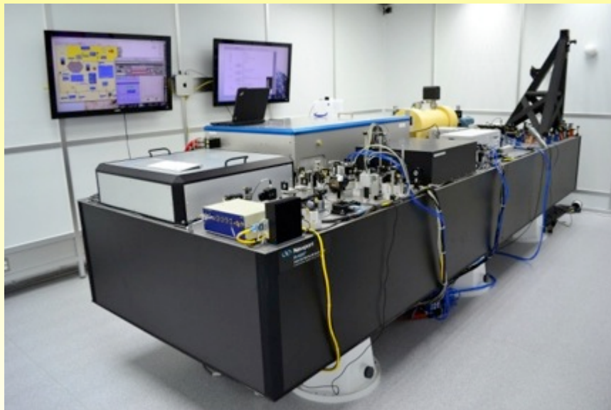
Installed Pre-Stabilized High Power Laser in the Laser Area Enclosure of the LIGO Livingston Gravitational Wave Observatory
