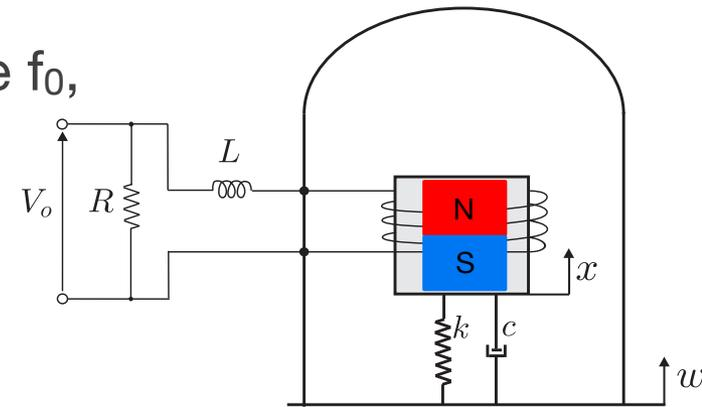
Figure 4: Working principle of a geophone.
