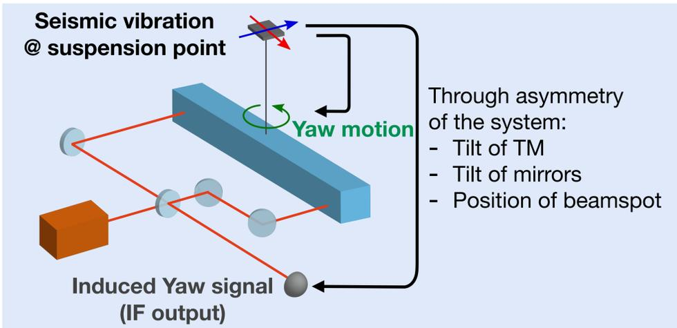
Seismic Cross-Coupling Noise = Seismic vibration  $\times$  Coupling Constant
