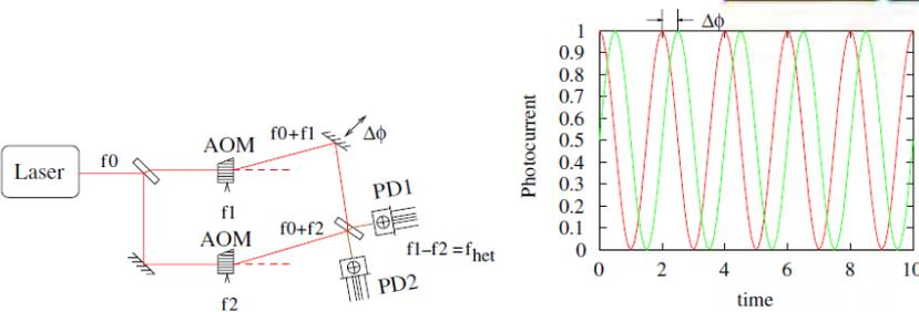
Figure 3. Heterodyne Mach-Zehnder interferometer: schematic (left) and typical photodiode signal (right).
