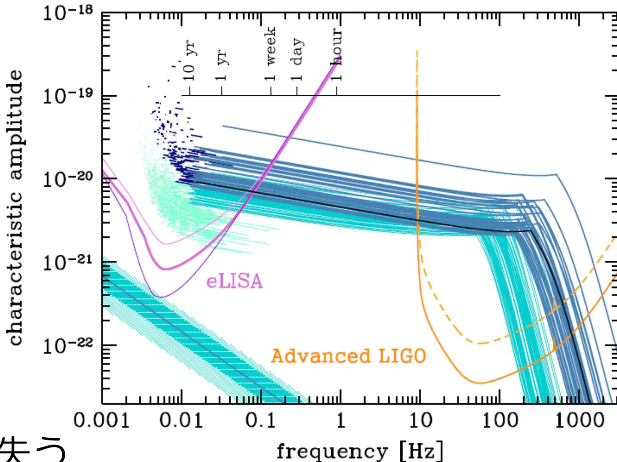
FIG. 1. The multiband GW astronomy concept. The violet lines are the total sensitivity curves (assuming two Michelson) of three eLISA configurations; from top to bottom, N2A1, N2A2, and N2A5 (from Ref. [11]). The orange lines are the current (dashed) and design (solid) Advanced LIGO sensitivity curves. The line
