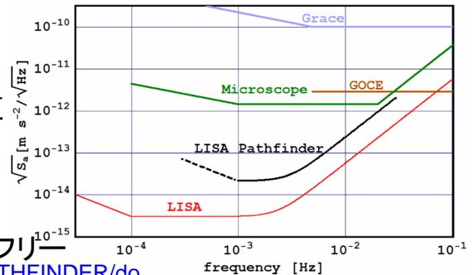
Figure 5: Comparison of required performances of various missions for relative geosismic deviation of test-mass pairs. For LISA Pathfinder the mission requirements are reported as the solid line. The dashed tail is a design goal. Actual projected performance is discussed later.
