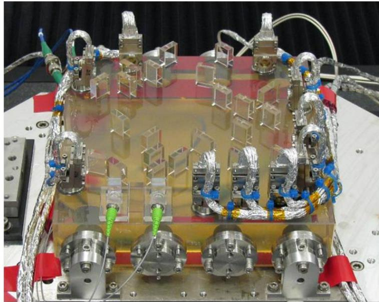
**Optical Bench Interferometer
