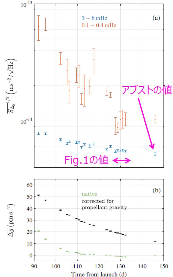
FIG. 3. (a) Square root of the averaged power spectral density of  $\Delta g$  in the 3–8 mHz and 0.1–0.4 mHz frequency bands of the time of flight. This is plotted for comparison with the noise level of the accelerometer. (b)  $\Delta g$  versus time from launch. The 'native' data is the raw data, and the 'corrected for propellant gravity' data is the data after correction for the gravity of the propellant. The 'Abstr. value' is the value of the 'Abstr.' data point at approximately 145 days.
