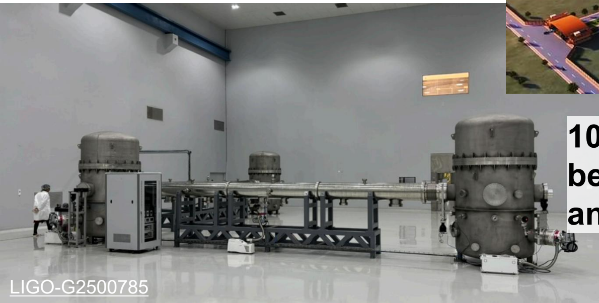
1:1 scale vacuum testing
