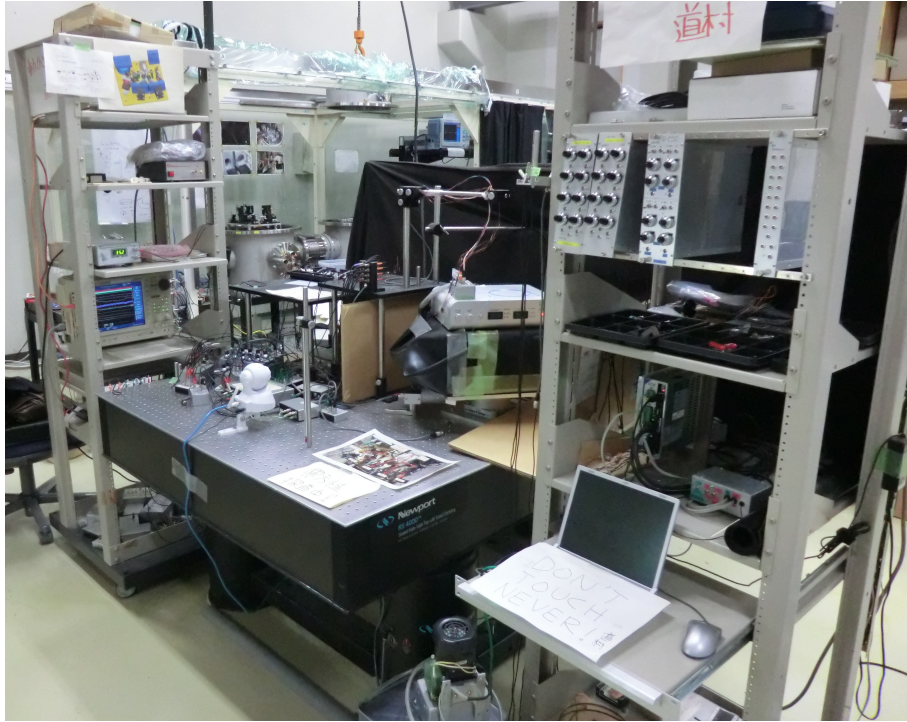
Figure E.1: The entire appearance of the apparatus. The vacuum enclosure on the turntable covered with black sheet is the main optical component, and the laser source is placed on top. Some electrical circuits and web camera are also put on the optical table. The rack on the left has the PZT driver and the data logger we used for the data acquisition. The rack on the right has the motor driver and the PC for controlling the motor for the turntable.
