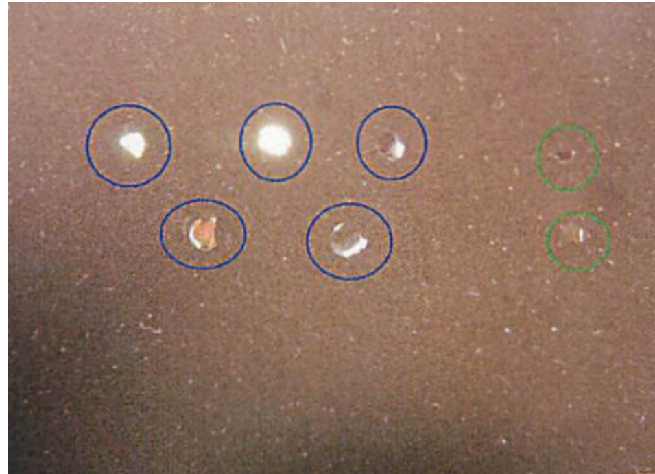
Picture of the mirror after coating. Only one of seven does not have any lack.
