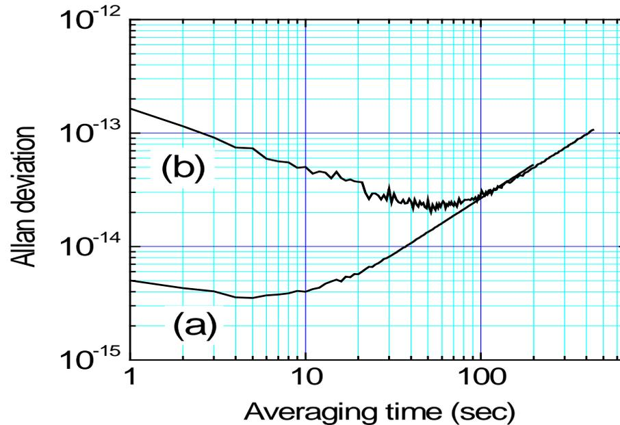
At NICT an optical frequency comb (femtosecond pulse mode-locked Ti:sapphire laser) was used to perform frequency stability measurements of an ultra-narrow linewidth 729nm clock laser.
