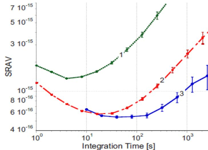
Beat between two nominally identical cryogenic sapphire oscillators; one oscillator acted as a reference oscillator with all control systems operational.
