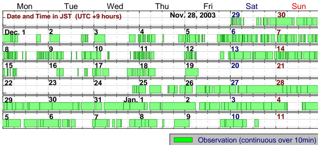
**Figure 3.** Operation status of the TAMA300 gravitational-wave detector during the ninth data-taking run (DT9) performed from November 28 in 2003 to January 10 in 2004. We operated the detector in the observation mode only at night and weekends in the first half; we spent most of the day time for tuning and characterization of the detector system. On the other hand, we operated the detector in full time with a high-duty cycle in the second half.
