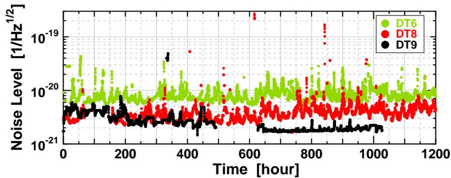
**Figure 5.** Stability of the noise level. Floor noise levels are plotted as a function of the time from the beginning of each data-taking run. There are diurnal changes in the noise levels in DT6, DT8, and the first half of DT9. On the other hand, the noise level is very stable in the second half of DT9.
