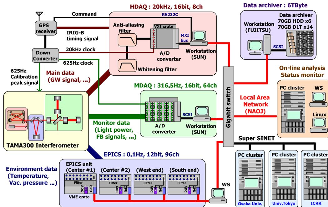
**Figure 2.** Data-acquisition system of TAMA300. Detector signals are recorded with HDAQ (20kHz, 8 channel), MDAQ (316.5Hz, 64 channel), and LDAQ (0.1Hz, 96 channel). The acquired data are sent to a data archiver, and recorded to DLT tapes. Stored data are distributed by a high-speed optical network connection.
