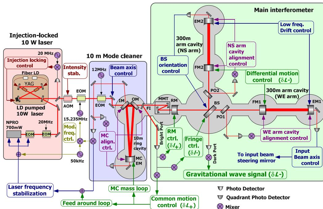
**Figure 1.** Optical and control design of the TAMA300 interferometer. TAMA300 is a Fabry-Perot-Michelson interferometer with a baseline length of 300 m and with power recycling. The laser source is an LD-pumped Nd:YAG laser with an output power of 10 W. A triangular ring cavity is inserted between the main interferometer and the laser source as a mode cleaner. The control system is designed to realize high sensitivity and stability of the detector at the same time.
