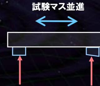
$$\delta\theta_d = \Delta\theta \frac{\delta x}{L} \quad \text{rad/Hz}^{1/2} \quad [\Delta\theta: \text{鏡の傾き}, \delta x: \text{並進変動}]$$
