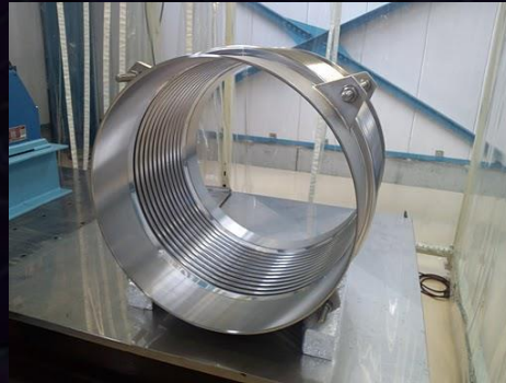
Bellows for each duct
