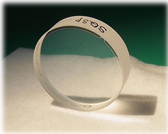
Figure 1: High quality mirror for KAGRA Figure 2: A picture of coating cross-section
