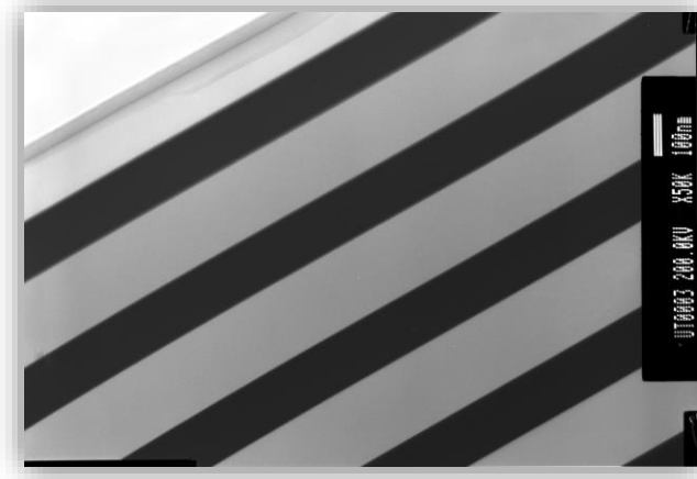
Figure 1: High quality mirror for KAGRA Figure 2: A picture of coating cross-section
