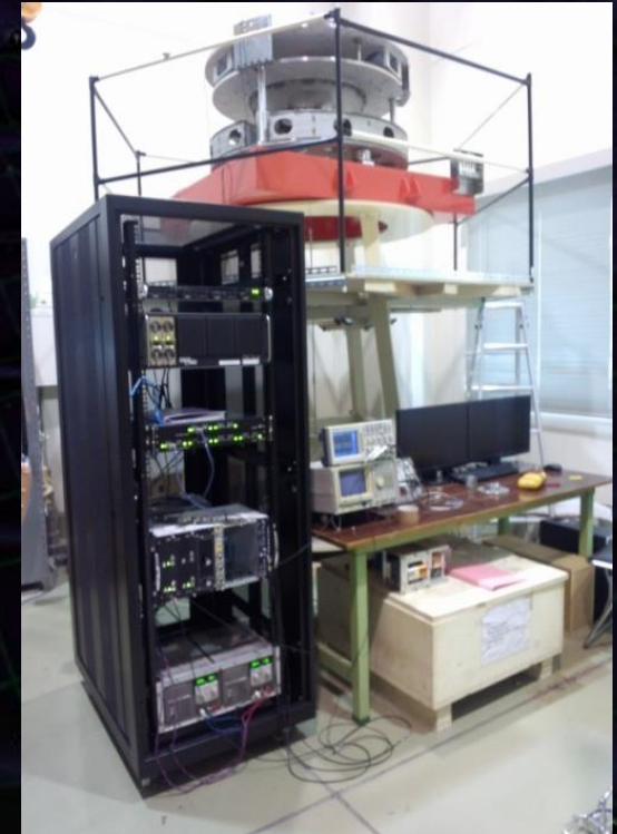
Control test of the pre-isolator prototype. The motion of the pre-isolator is controlled by the digital system mounted in the rack.
