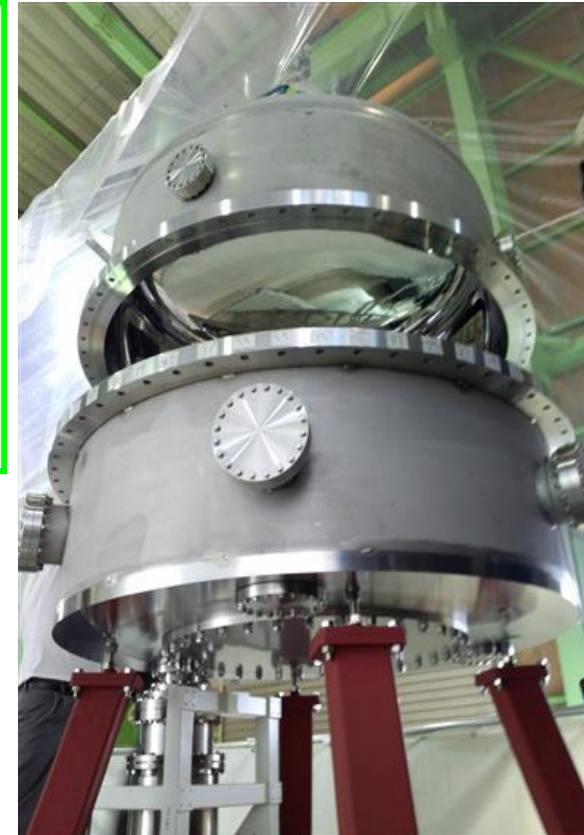
Leak test of the \phi 1500 chamber in which the pre-isolator is put away. Metal O-rings are used to seal the flanges.
