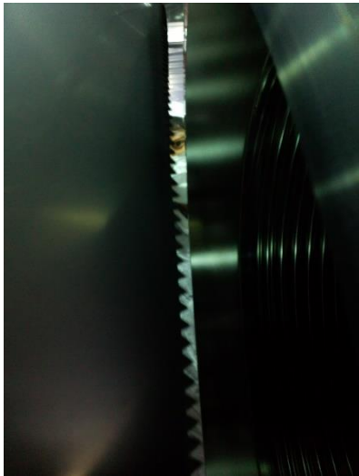
Prototype of shading baffle inserted into \phi 800 tube. The baffle has saw shape edge.
