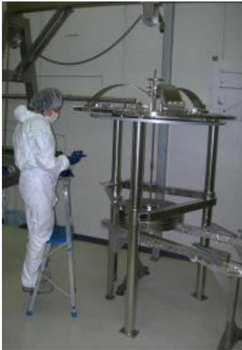
Tuning of the top filter. The natural frequencies were tuned to 0.2Hz.
