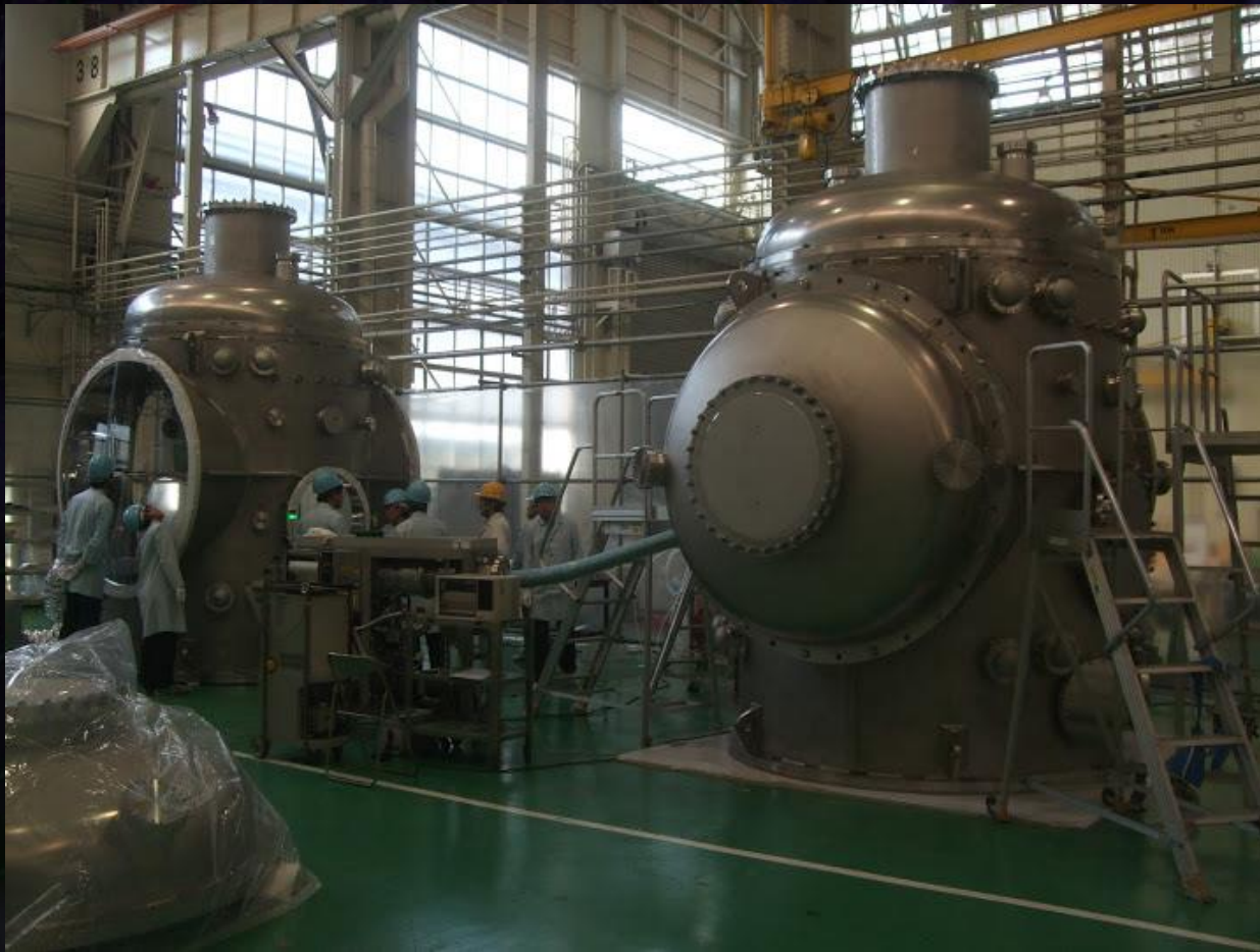
Cryostat #1 in preparation for installation of radiation shield.
