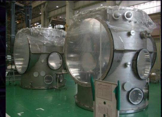
3 rd and 4 th cryostats under construction
