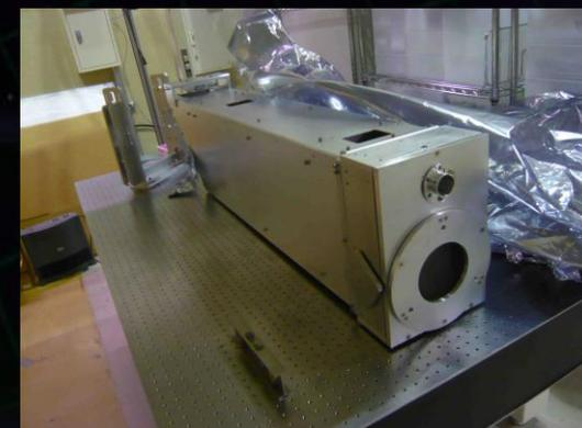
透過光用Beam reducing telescope
