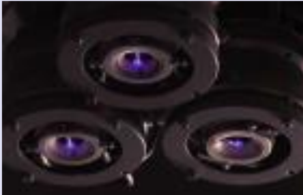
Needle Type FEEP ( \sim 10\mu\text{N} ) : flight proven
